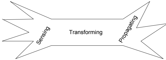
Fig. 1 Monitoring node (basic functions: different sensing and propagating sub-functions can be used for information transfer from and to nodes of external (to monitoring node) information logistics environment); each sensing sub-function can be viewed as having soft or hard sensors depending on whether it is performed by humans or artificial performers [6].
